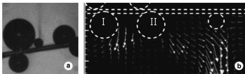
Fig. 10. Effect of bubble size on jet flow. (a) CCD image; (b) PIV measurements.
